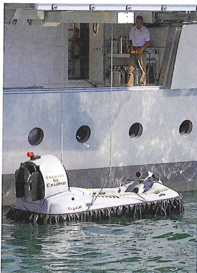
right Stowage for the extensive toy collection is particularly impressive, with various compartments housing everything from an amphibious car to a Hov Pod hovercraft, both launched by beam cranes in the hull sides.
